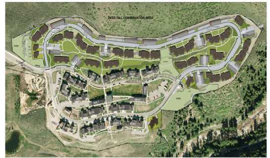
2. ILLUSTRATIVE BURLINGAME RANCH AFFORDABLE HOUSING PROJECT PHASE II MASTER PLAN. A strong, central pedestrian core of open space and public facilities connects growth and interaction, while vehicular circulation and "curb-to-curb" facilities are reduced to the outer loop road. A series of shared pedestrian paths and public pedestrian destinations is also in place to connect each building that connects to Aspen and other destinations. The building is oriented with the topography to minimize the size of the walls and provide good views from each side. Canopies are used to shade porches on the left side of the loop road and incorporate an additional 50 square feet of outdoor storage for each unit. Specially designed trash enclosures, transit stops and mail centers are also integrated into the plan as components of the supports and are evenly distributed throughout the site to maximize proximity to the residents.
