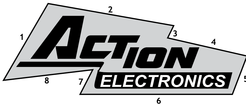
Figure 13-2: For irregularly shaped signs, area is measured as enclosed by up to 8 straight intersecting lines.
