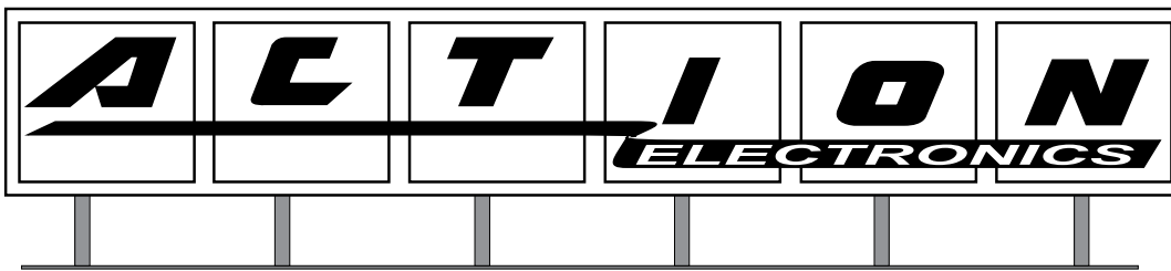
Figure 13-5: Sign area must include vertical and horizontal spacing between letters conveying the sign's message.
