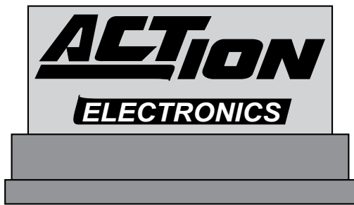
Figure 13-3: Sign area for a monument sign must not include base, if the base is architecturally distinct.
